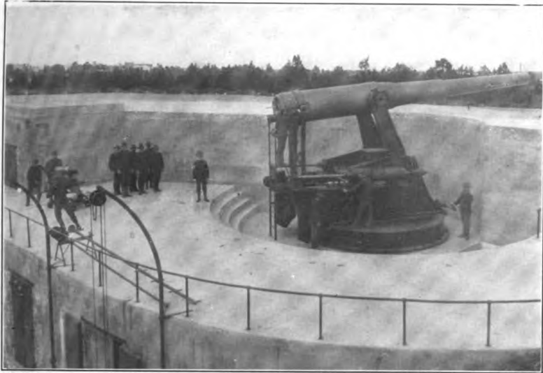
FIG. 1. Gun Mounted on 10-inch Disappearing Carriage, Model 1896, the Instant before Firing. Gun rises to this position in about six seconds.
