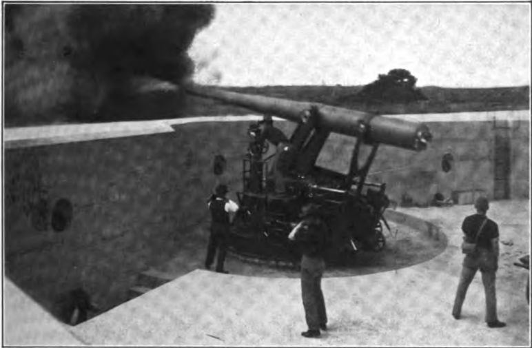
FIG. 1. Six-inch Disappearing Carriage, Model 1898. (Photograph taken during recoil about 1.10 second after firing. The dark cloud is mainly dust from the parapet.)
