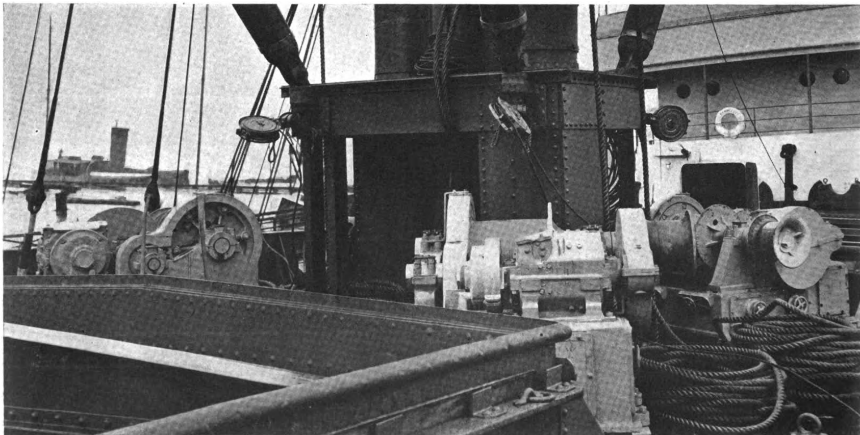
Three of the Allan-Cunningham-General Electric motor-winchs on the deck of the "Kennecott"
