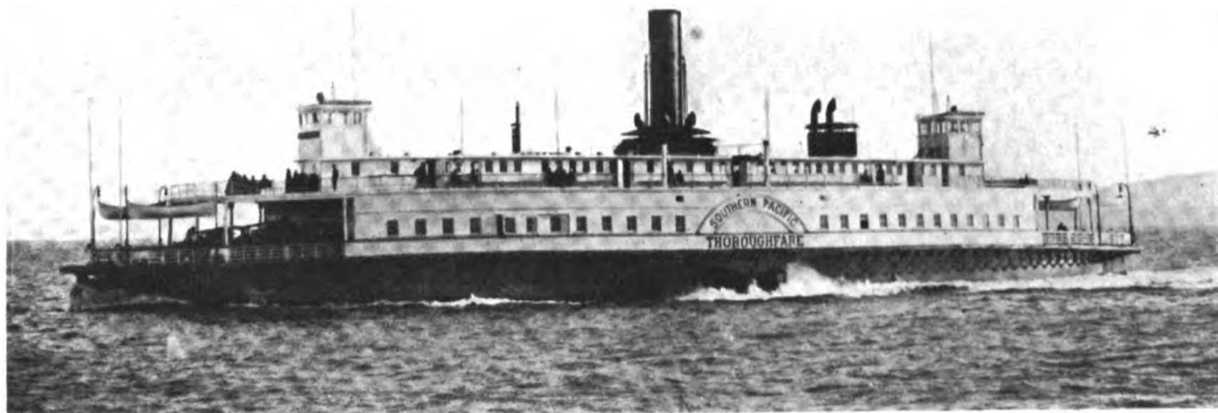
Type of ferry used in Frisco Bay, now steam-driven but likely to be converted to Diesel-electric power.
