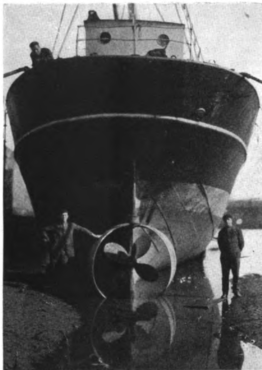
Depicting Kitchen reversing-rudder on stern of Diesel coaster "Alca"
