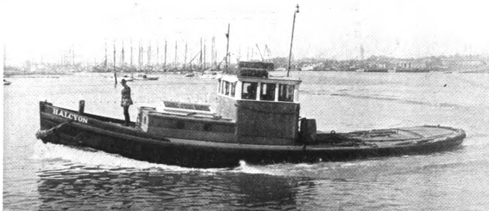
Motor-tug "HALCYON" now powered with a 125 b.h.p. Atlas Diesel engine, the old Atlas distillate engine having been removed for economy purposes.
