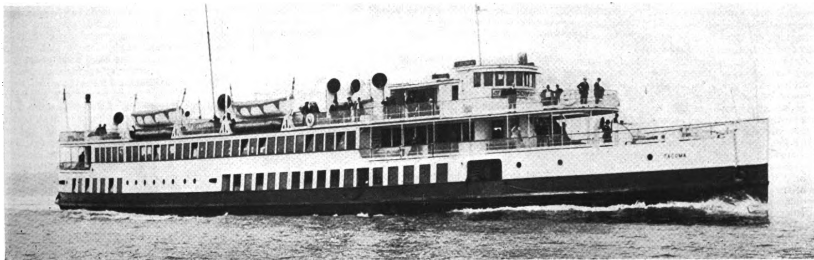
"Tacoma," one of the Puget Sound Navigation Co.'s steam-driven ferry on the run between Seattle and Tacoma. We have painted-out the smoke stack to show how their new 18-knot Diesel-electric ferry vessel will look. This company operates 20 steamers and as soon as practicable will convert them to Diesel or Diesel-electric power
