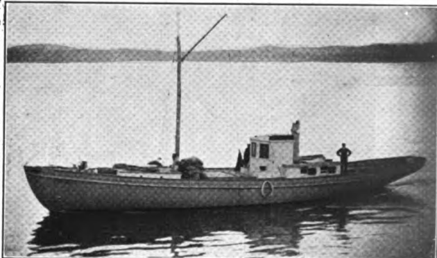
"Patriot," owned by Booth Fisheries Co. Has 60 h.p. surface-ignition oil-engine
