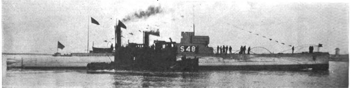
New U. S. Navy 1,000 tons surface-displacement submarine "S-48" launched by the Lake Torpedo Boat Co., Bridgeport, on Feb. 26th. She is propelled by a pair of 950 b.h.p. Busch-Sulzer Diesel-engines. Her length is 240 ft, and she carries one 4-in. gun and has five 21-in. torpedo tubes.
