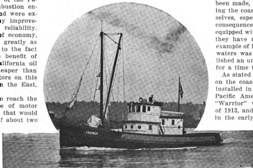
"Chomly," the record Pacific Coast Cannery tender to be Diesel-powered. Like the "Warrior," and "Chickamauga" she has Nelseco engines
