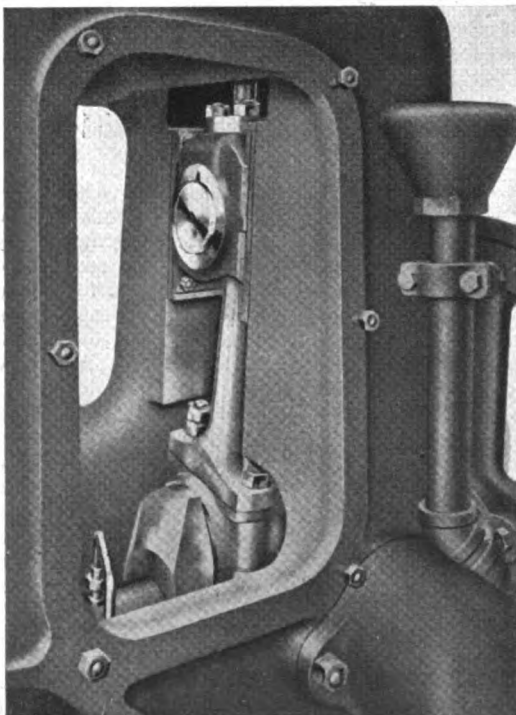
Looking through door in crank-case frame, showing crosshead and guide
