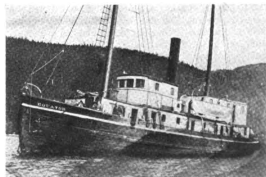
"Equator," one of the steam tugs of the Carey-Davis Tow Boat Co., Seattle, which will be changed to Diesel power. A 300 h.p. engine will be installed
