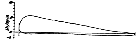
SCAVENGING CARD SPRING 1'' = 15 \text{ LBS/SQ. IN.} TAKEN AT THE SAME LOAD AS THE WORKING CARD ABOVE.
