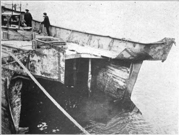
A BRITISH TRAWLER WITH BOW BLOWN OFF BY A MINE
