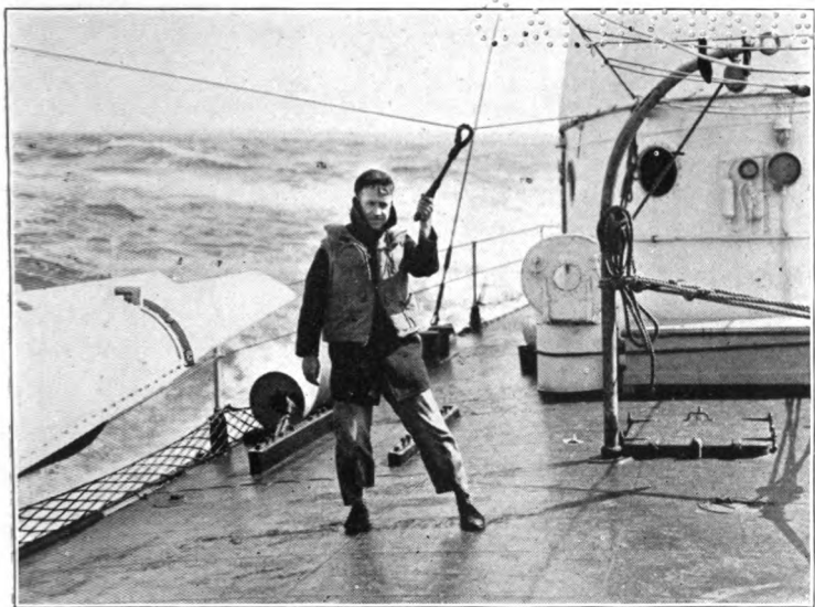
LIFE LINE ALONG THE DECK OF AN AMERICAN DESTROYER IN READINESS FOR ROUGH WEATHER
