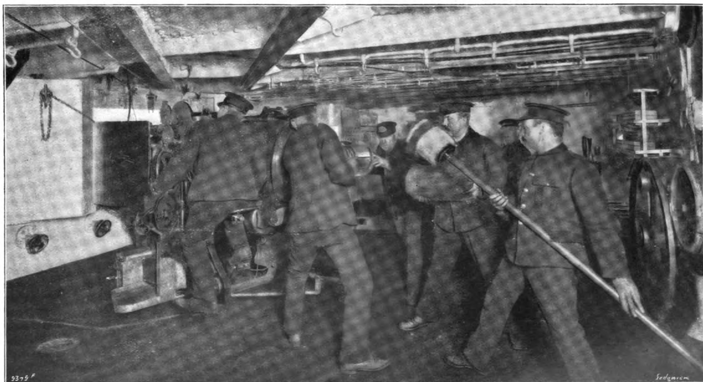
FIG. 10. LOADING 6 IN. QUICK-FIRING GUN.
