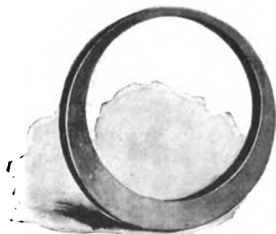
SECTION OF AN IMPERFECT CAST IRON STEAM PIPE.
